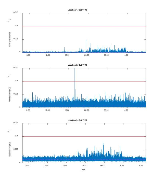
Figure 1: RMS particle accelerations at Location 1, 2 and 3 on October 17-18, 2017. The magenta dash line represents the mean baseline rms particle acceleration calculated from October 5 to 16 at each location. The red line shows the  $0.01 \, \text{m/s}^2$  threshold of the RMS particle acceleration.
